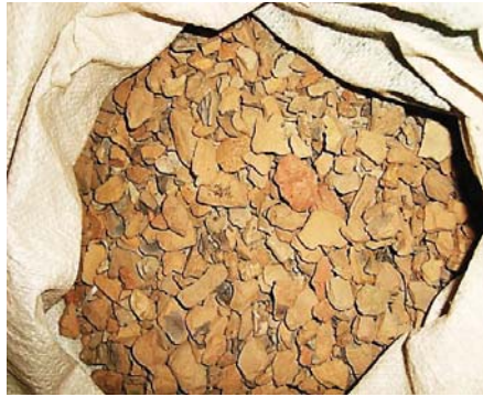
FIGURE 2. Artificial lightweight aggregates [18,22,23].
