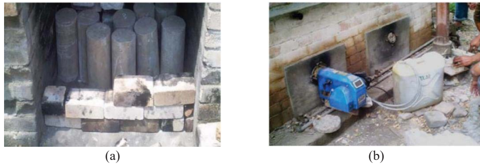
FIGURE 2. The fire test: (a) the concrete specimens inside the furnace, (b) burner setup.
