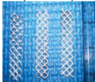
FIGURE 1. Aluminum fiber with 10 mm x 25 mm dimension produced from aluminum net waste.
