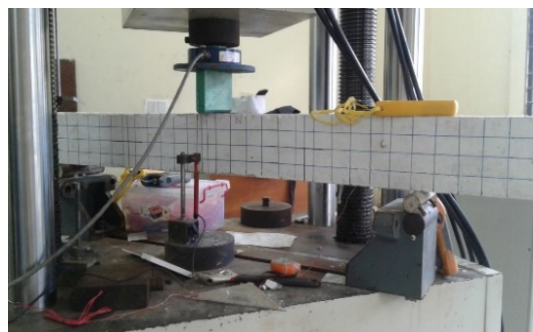
Fig. 6 Three-point bending test for RC beam
