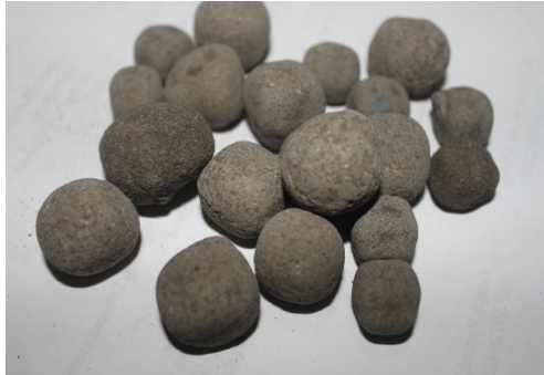
Fig. 3 Polypropylene waste coarse aggregate coated with sand
