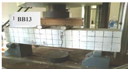
(b) Beam bamboo with mortar M13 (BB13)
