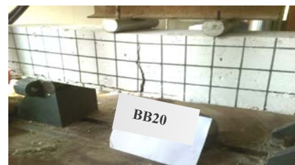
(c) Beam bamboo with mortar M20 (BB20)
